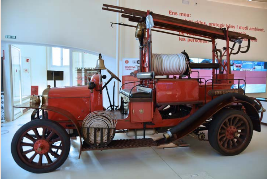
Delahaye 84 PS - Genoveva engine. Bought in 1923. Made in France. Lightweight fire engine with a 400-litre water tank for self-sufficient firefighting. ABB
