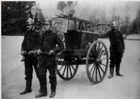
MTM 1875 pump. Bought in 1875. Hand fire pump manufactured by Maquinista Terrestre i Marítima based on a French model. For drawing water directly from a pond or canal. It has a tank which can be filled with buckets of water. ABB
