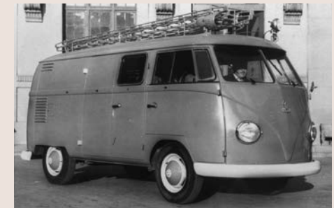
W BT 19 1955. Bought in 1955. Volkswagen T1 van fitted out by Rosembauer with a high-pressure pump to put out small fires. It would be used at the fire station inside the Barcelona Trade Fair facility. ABB. The van at the exhibition belongs to Marcos Navarro's private collection.
