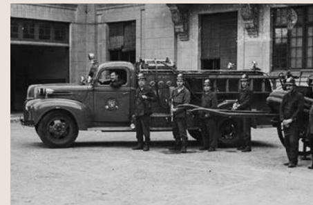
Bt7 1948. Bought in 1948. United States Army surplus war equipment. Truck specially designed to fight fuel fires at airfields. ABB
